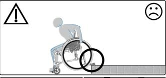
The anti-tipper must be deactivated when moving down over edges.
