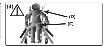
The seat belts must not be twisted during use or passed over components and thus kept away from the body. They have to be tight and tight without compromising user comfort. The lap belt buckle must be between the pelvic bones (as centrally as possible). The buckle tongues on the lap belt for fastening the shoulder belt should be on the outside of the pelvis, if possible.
