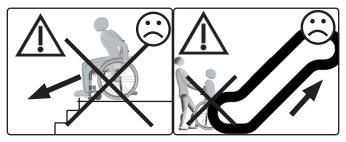
Conquer stairs only with the help of experienced helpers. To do this, the anti-tipper must be deactivated. Always carry the wheelchair by the frame, never by the seat shell, the pull-out push handles / push bar, the legrest and / or the footplate (s)!
