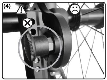
The anti-tipper must always be locked in its end position.
