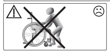
Do not use the footplate to get in and out. The wheelchair could tip forward.
