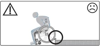
The anti-tipper must be deactivated when driving down on edges.
