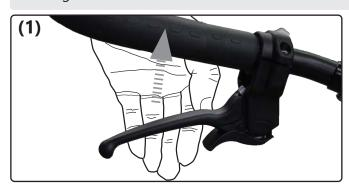
Uneven use of both brake levers causes cornering.
