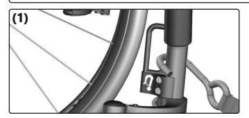
The wheelchair must be attached using a vehicle-anchored 4-point wheelchair restraint system in accordance with ISO 10542. These can be snap hooks, S-shaped hooks or snap fasteners. The wheelchair restraint system must be securely attached and used in accordance with the manufacturer's instructions for use. (3A+B)
