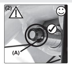
After each insertion, pull at least once to test whether the quick-release axle is engaged. It must no longer be possible to pull the wheels outwards.
