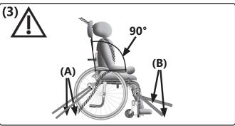
If the wheelchair is equipped with a back angle adjustment or seat tilt, it must be ensured that the occupant sits in an upright position with a back angle of 90 ° during transport (3). Legrests that can be swiveled up must be set to the lowest position.
