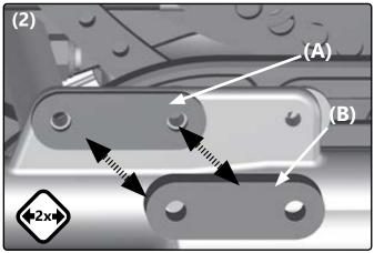
Correct the quick-release axle fittings and turn them out/in so far that the tire of the wheel is as little as possible at the crest, but at least 8-10 mm away from the side part or the clothes guard (see chapter "Wheel assembly").
