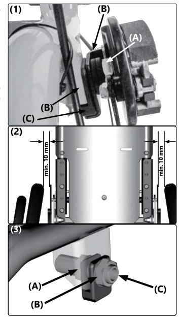
$\triangle$  After adjusting the quick-release axle adapter, be sure to check that the wheel lock functions properly.
