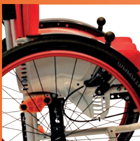
brake integrated into the clothing guard side parts
